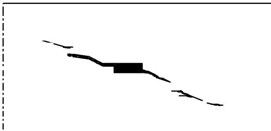
Fig. 1 of C(2011) - Shear failure by the asymmetric four point bending test with small center-slit. (Sketch after a photo)
